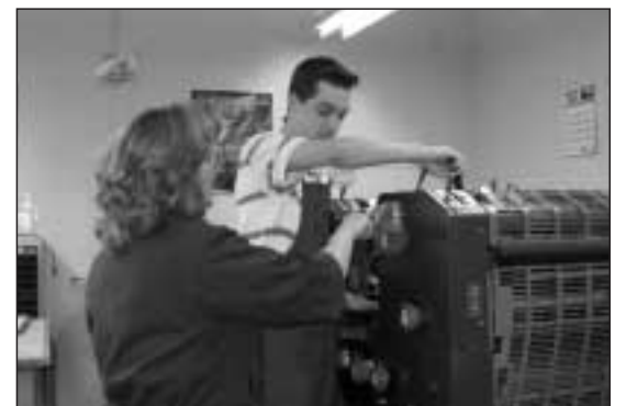
Justin Bowen, a student at SCCTC, sets up the A.B. Dick 9995 to print a four-color process job.
